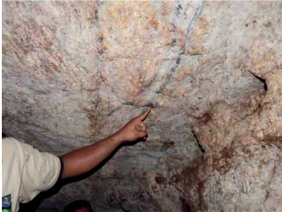
Figure 21: Graphite veins showing in an old adit in COM 011
