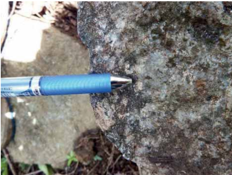
Figure 26: Close up of graphitic quartz feldspar rock close to old shafts in EL954
