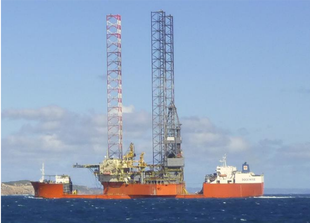
West Telesto drilling rig on transport ship
