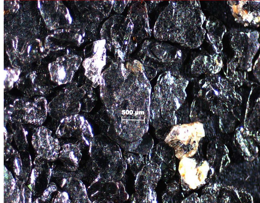
Final concentrate showing coarse nature (Test No. GK 18)
