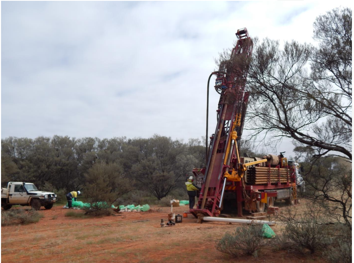
Figure 2: Reverse circulation (RC) drilling of Australian Mines' priority nickel, copper and gold targets has recently commenced at Marymia. This drill campaign, which initially comprises 11 RC holes, is scheduled to take five weeks to complete.
