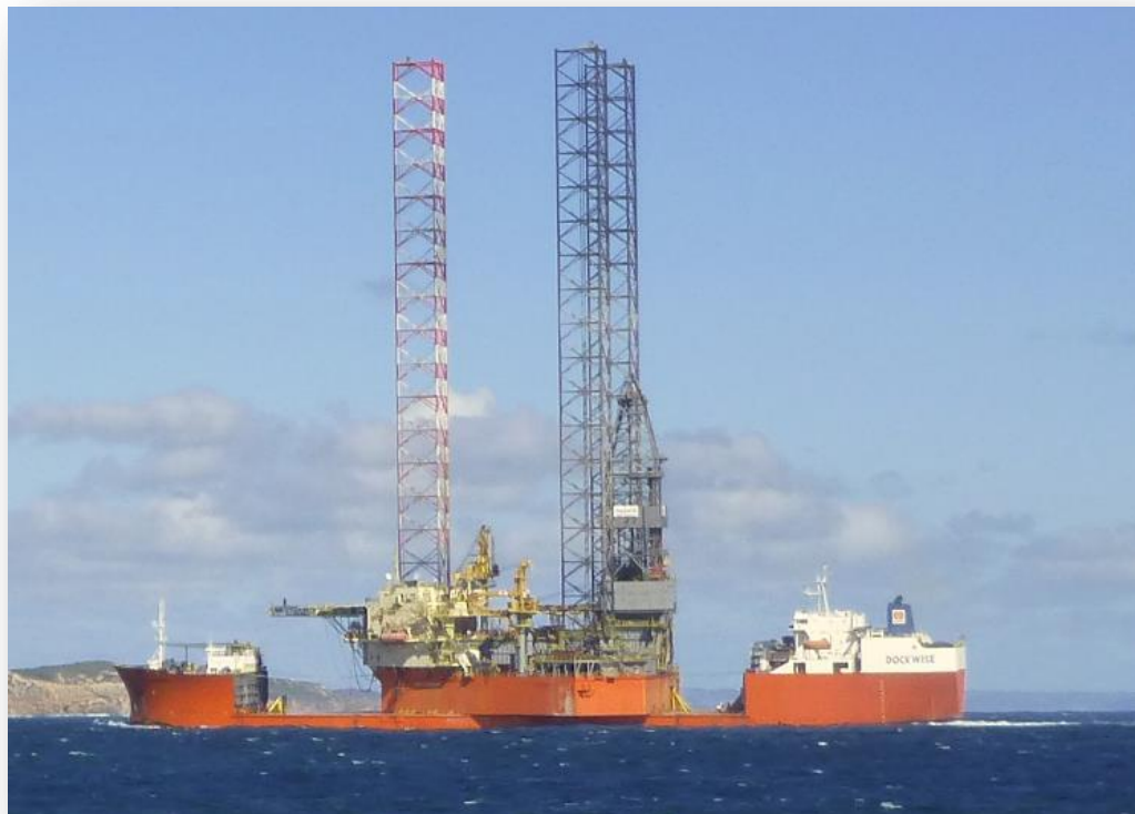
West Telesto drilling rig on transport ship
