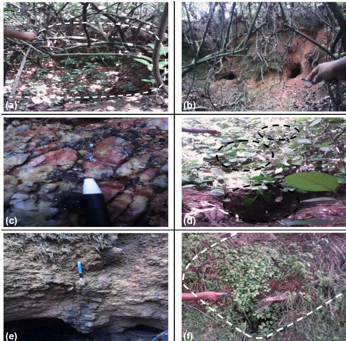
Figure 2. Abandoned Graphite mine site 4 in Grid 34 (a) Partially filled shaft covered by thick Diyapara vegetation (b) Two adits opened to the main Shaft (c) Graphite flakes associated with Quartzite (d) Interconnected series of adits (e) Graphite associated with a pelitic band going through laterite observed at adit mouth (f) A shaft totally filled with debris.
