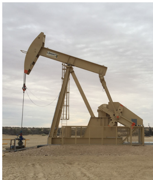
Beam pump installation at Callawonga-7
