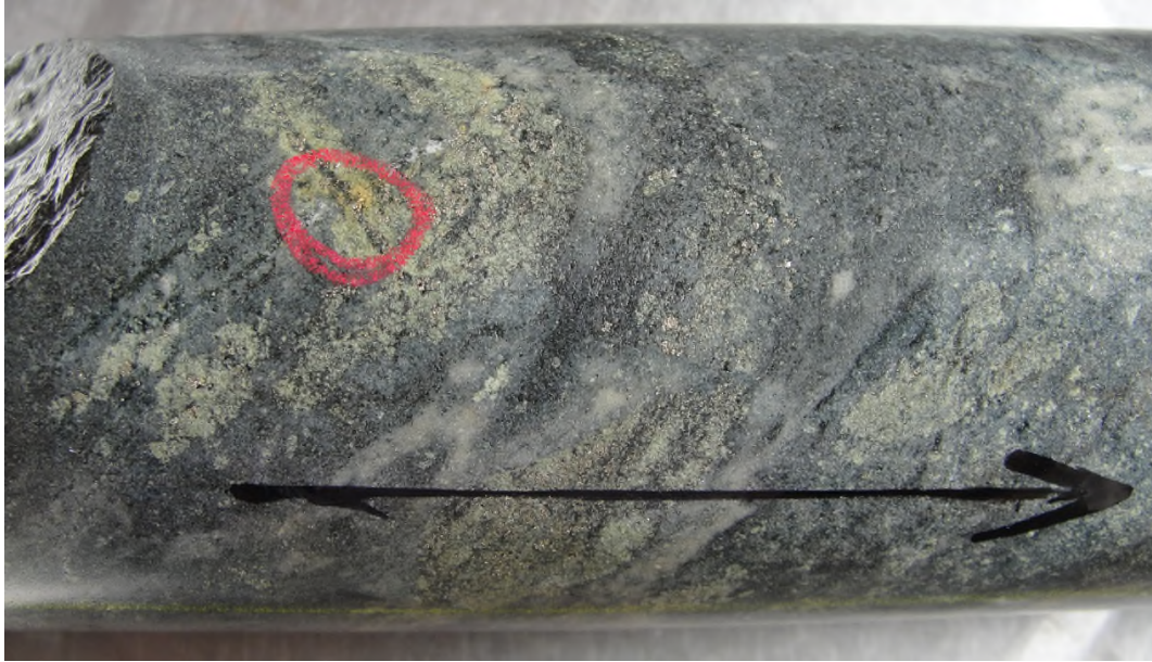
Figure 2. Specks of free gold at the intersection of two cross cutting fractures in GRDD003. Note association of strong silicification and disseminated pyrite.
