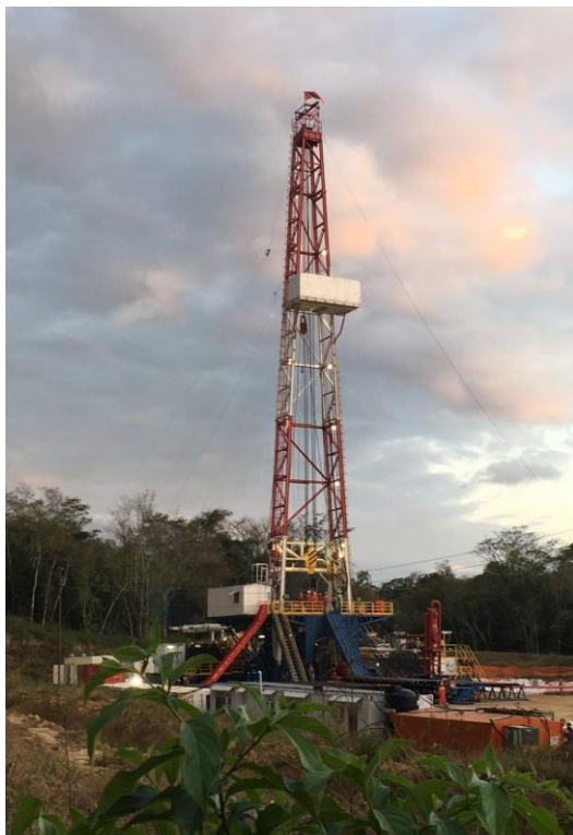
Pictures (left and above): Drilling operations of the MD 250 well using 4,000m rig
