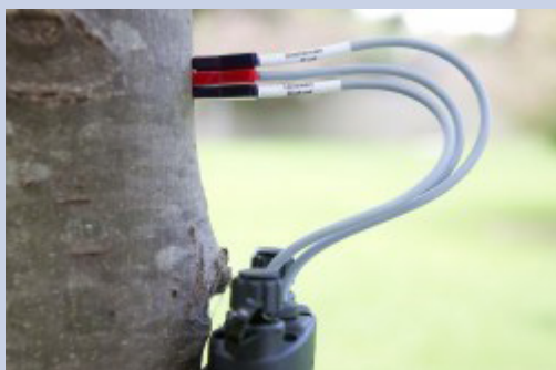
Special equipment is used to measure how much and when water is used by the almond trees (left) while the 'Stem Psychrometer' (right) measures plant stress
