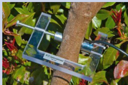
Special equipment is used to measure how much and when water is used by the almond trees (left) while the 'Stem Psychrometer' (right) measures plant stress
