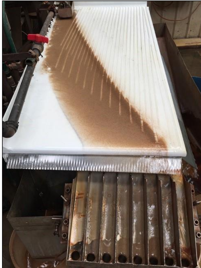
Figure 3: Wilfley Table Test
