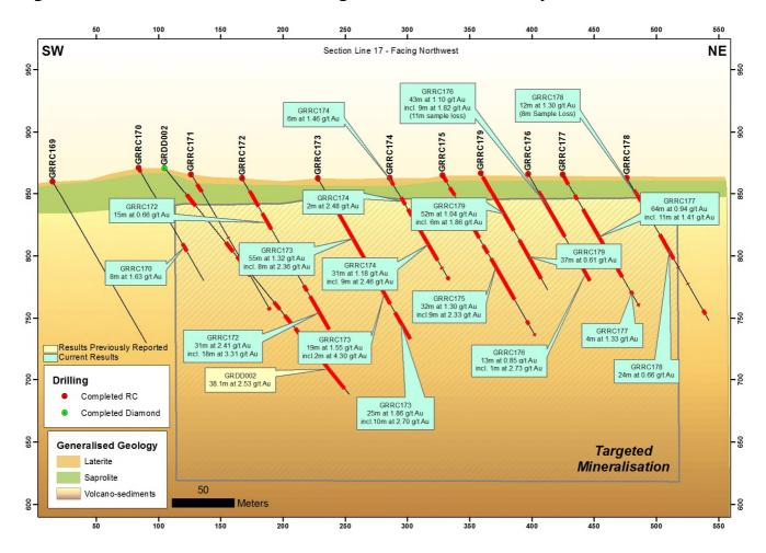
Figure 3: Section across Line 17 showing the mineralised intercepts over 400m
