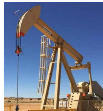
Variable speed beam pump installation in ex PEL 91
