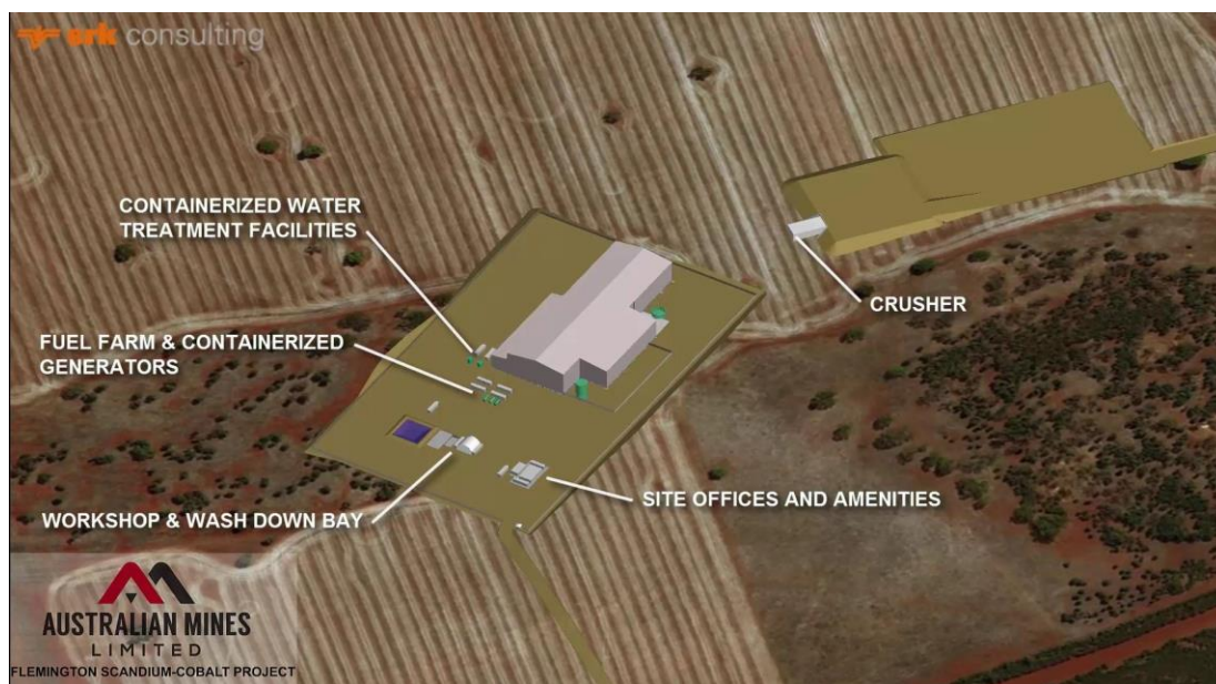
Figure 2: Schematic image showing the proposed footprint of the infrastructure at the Flemington mining operation.
