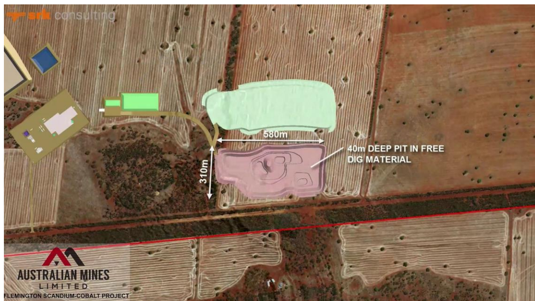
Figure 1: Proposed design of the open pit mine at Flemington. Indicative location of the processing plant shown to the west of the proposed mine. The area shaded in green to the immediate north of the proposed pit represents the area to be drilled at part of the Australian Mines' upcoming resource extension drill program targeting high grade cobalt and scandium mineralisation.
