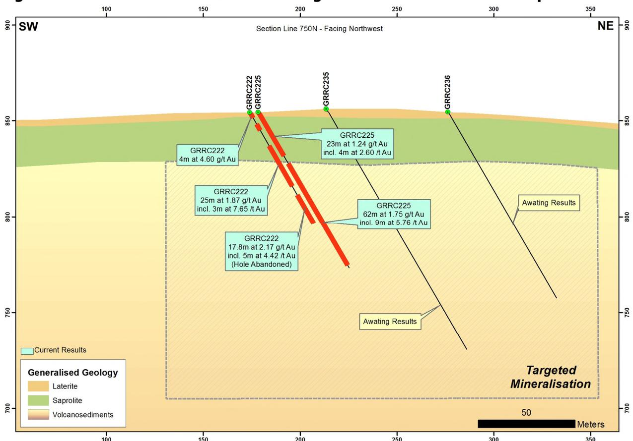
**Figure 3: Section across Line 750N showing the main mineralised intercepts**
