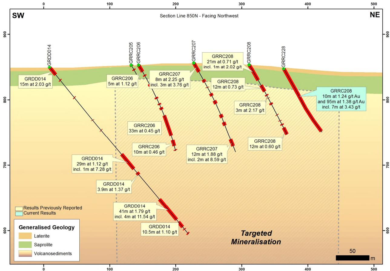
**Figure 4: Section across Line 850N showing the main mineralised intercepts**
