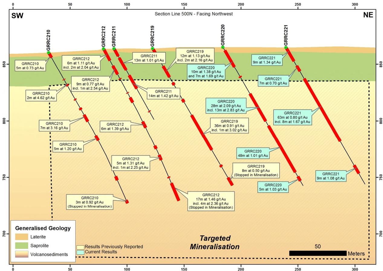
**Figure 2: Section across Line 500N showing the main mineralised intercepts**
