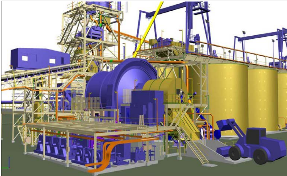
Figure Two: Dalgaranga Processing Plant – SAG Mill and CIL Tank Layout
