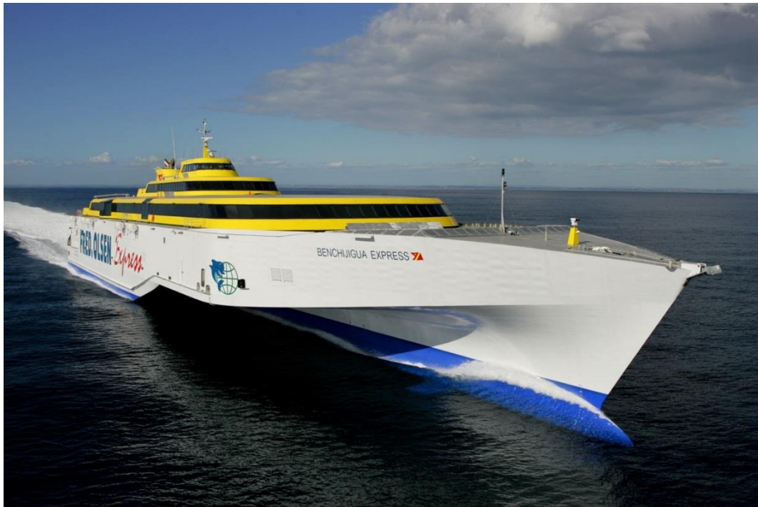
The 127m Benchijgua Express was the world's first and largest trimaran hull vehicle passenger ferry, designed and built by Austal for Fred Olsen S.A. in 2005. (Image: Austal)
