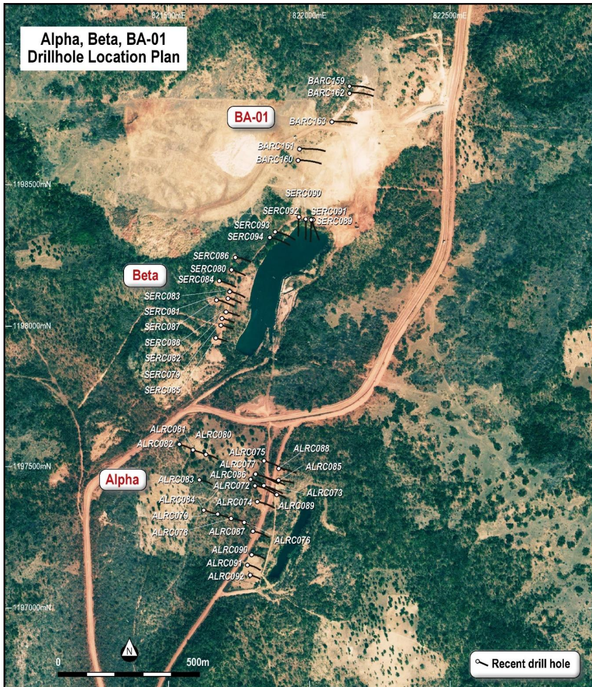
Figure 4: Surface plan showing recent drilling at the Alpha, Beta BA01 satellite deposits
