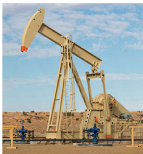
Artificial lift installation post Bauer Field pad drilling.
