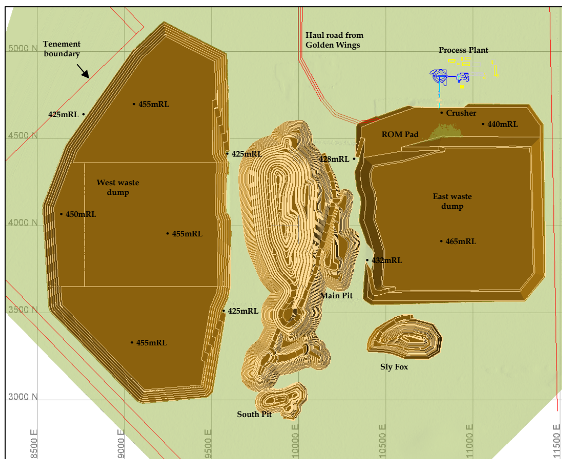
Figure B7: Gilbeys – Final Waste Dump Designs
