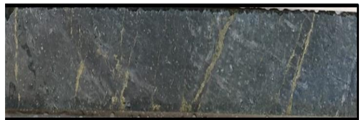
Kadungle Project (above) - Drill hole KDD017 with sheeted chalcopyrite \pm pyrite veins assaying up to 1.63% copper and 0.12g/t gold
