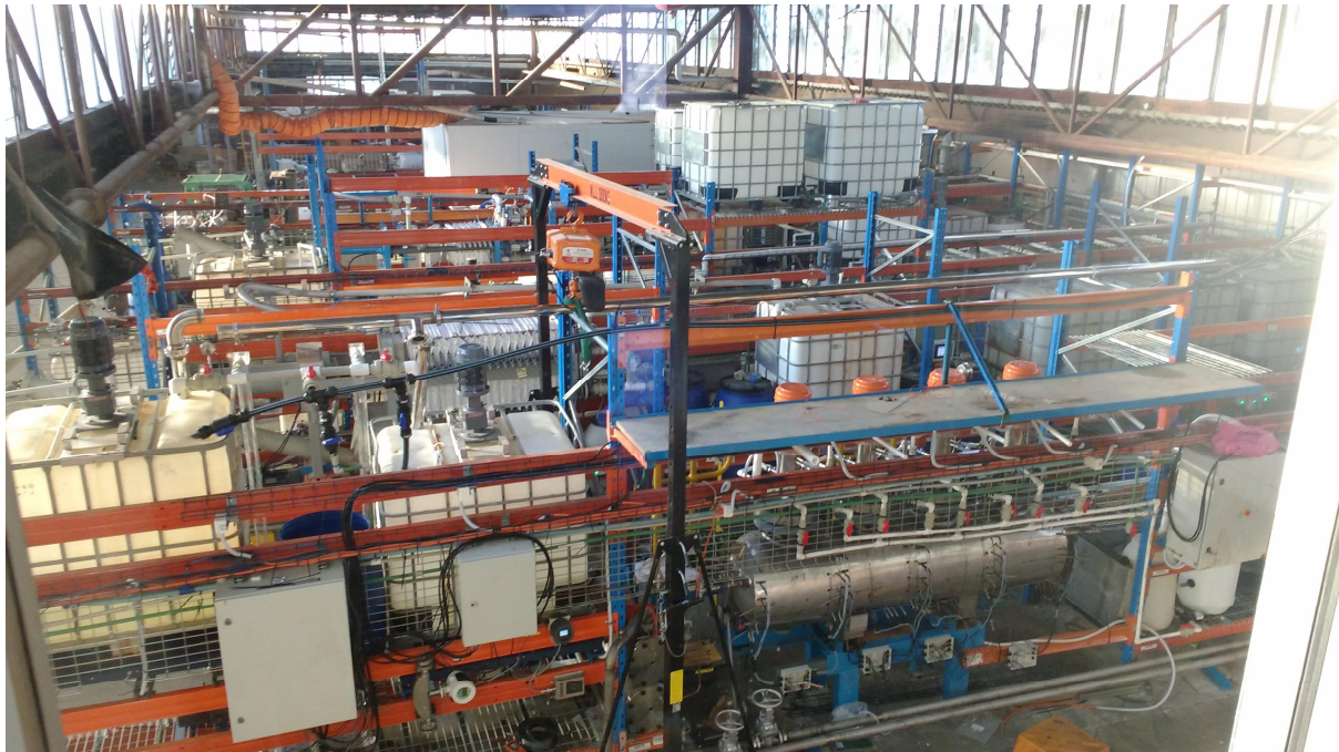
Figure 3: The Demonstration-scale processing plant is a 1:2,500 scale of a commercial 2 million tonne per Pressure Acid Leach + Solvent extraction processing plant. The demonstration-scale plant is located in Simulus Laboratories facilities in Welshpool, Western Australia.
