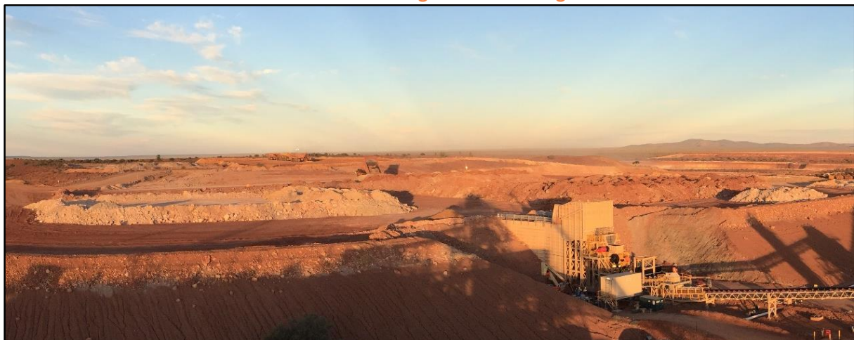
Photo 8: ROM Ore Stockpile being developed ahead of Processing
