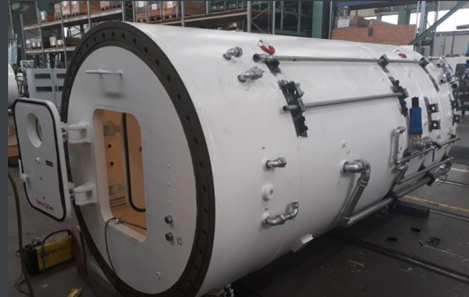
West Gate Tunnel Project TBM personnel lock and cutter head being manufactured in Germany
