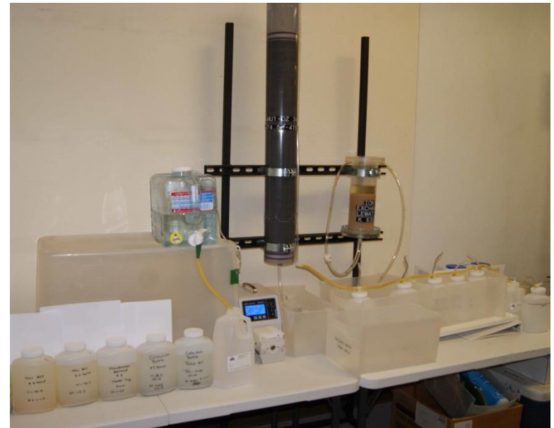
Column Leach Test Apparatus at Lance
