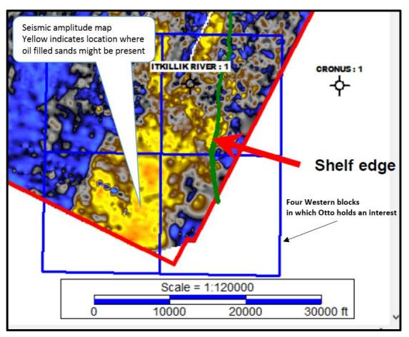
Exploration success in the Nanushuk play-fairway is now being driven by the understanding that when reservoir quality top set sands are present anomalously high amplitudes are seen on seismic data.
