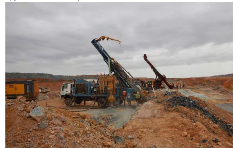
Pre-collar drilling (foreground), diamond tail drilling (background) – Rosemont South
