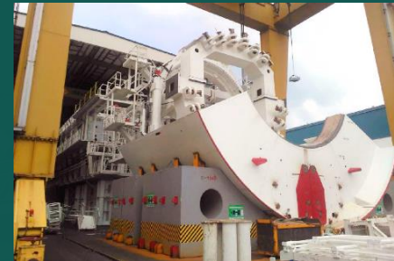
TBM shield under construction
