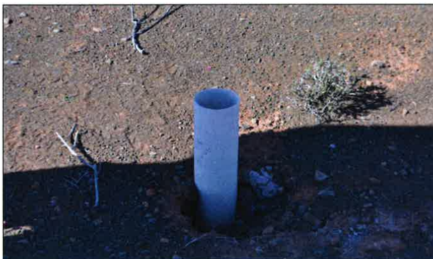
Figure 5-7: Drill hole casing of a borehole at Ryst Kuil
