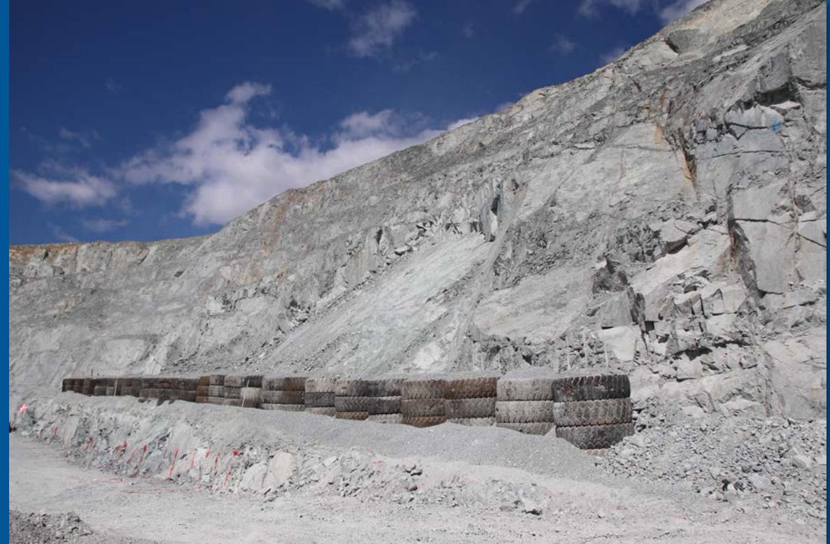
Innovative tyre bund for ground control at Mt Rawdon
