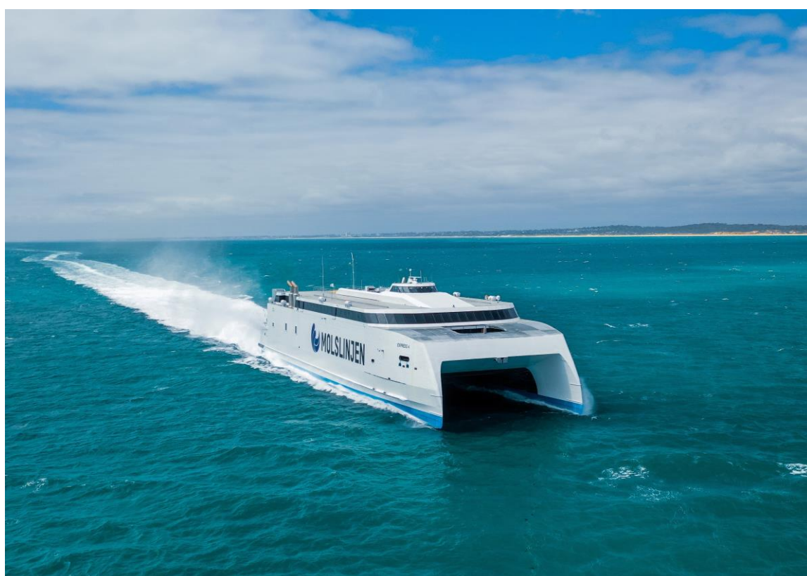
Molslinjen Express 4 achieved in excess of 40 knots during high speed trials off the coast of Western Australia, January 2019 (Photo credit: William Blaauw)
