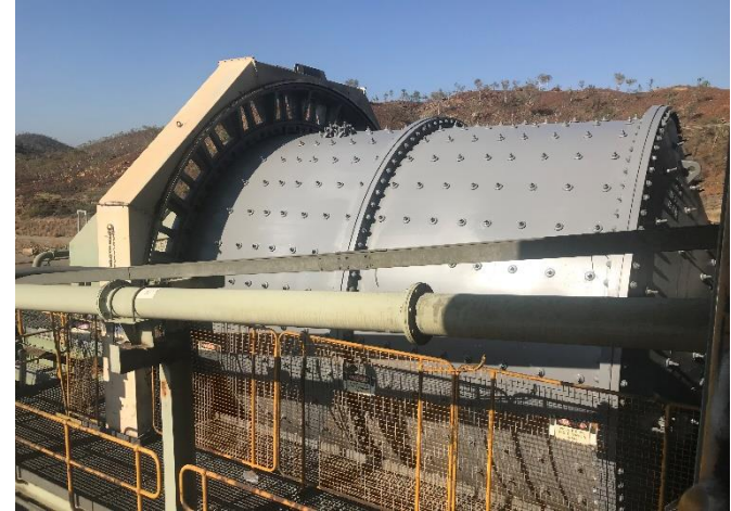
Refurbished SAG Mill
