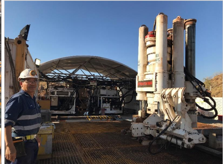
Savannah North raise bore rig and platform
