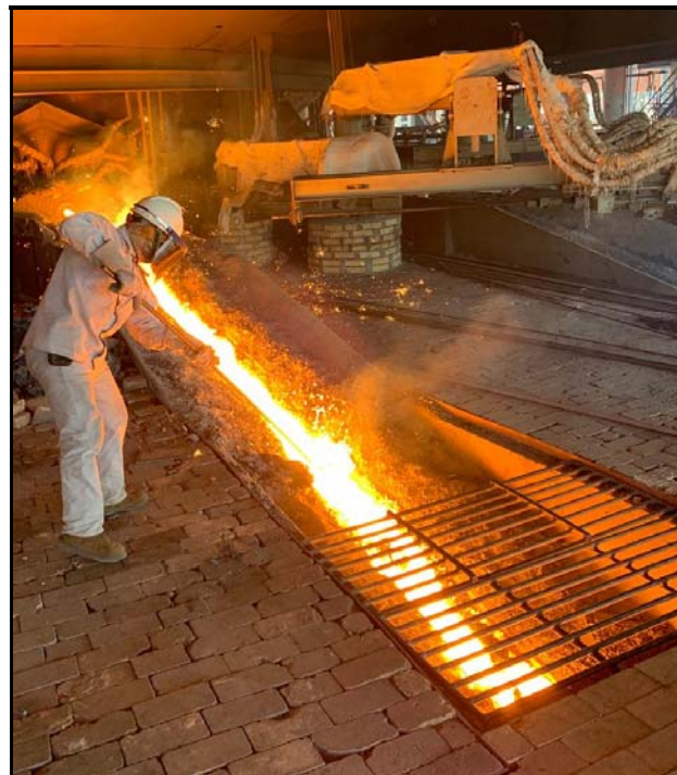
The second Hengjaya Nickel kiln being tapped for NPI
