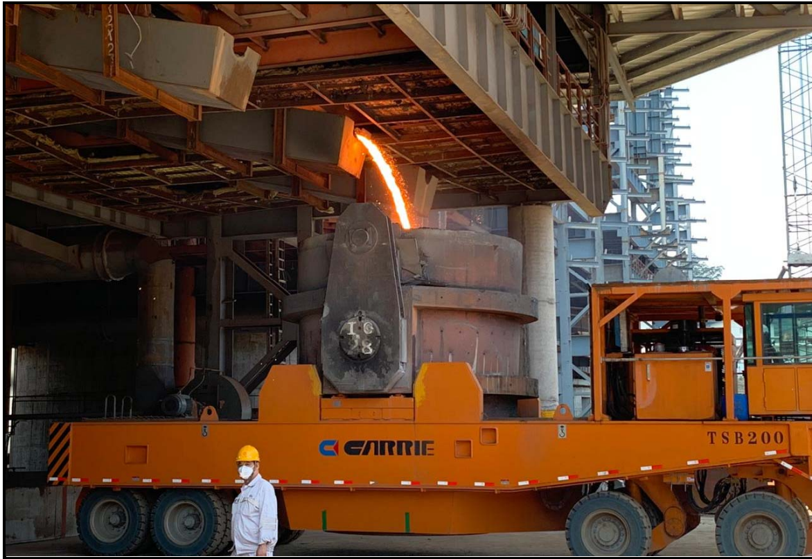
NPI being poured into a crucible for direct hot transfer into IMIP stainless steel lines
