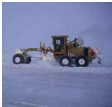
Ice roads enable essential equipment and supplies, including drill rigs, to be mobilised to site during winter. The roads melt in spring, leaving minimal impact on the sensitive tundra.
