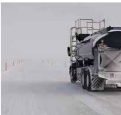
Ice roads enable essential equipment and supplies, including drill rigs, to be mobilised to site during winter. The roads melt in spring, leaving minimal impact on the sensitive tundra.
