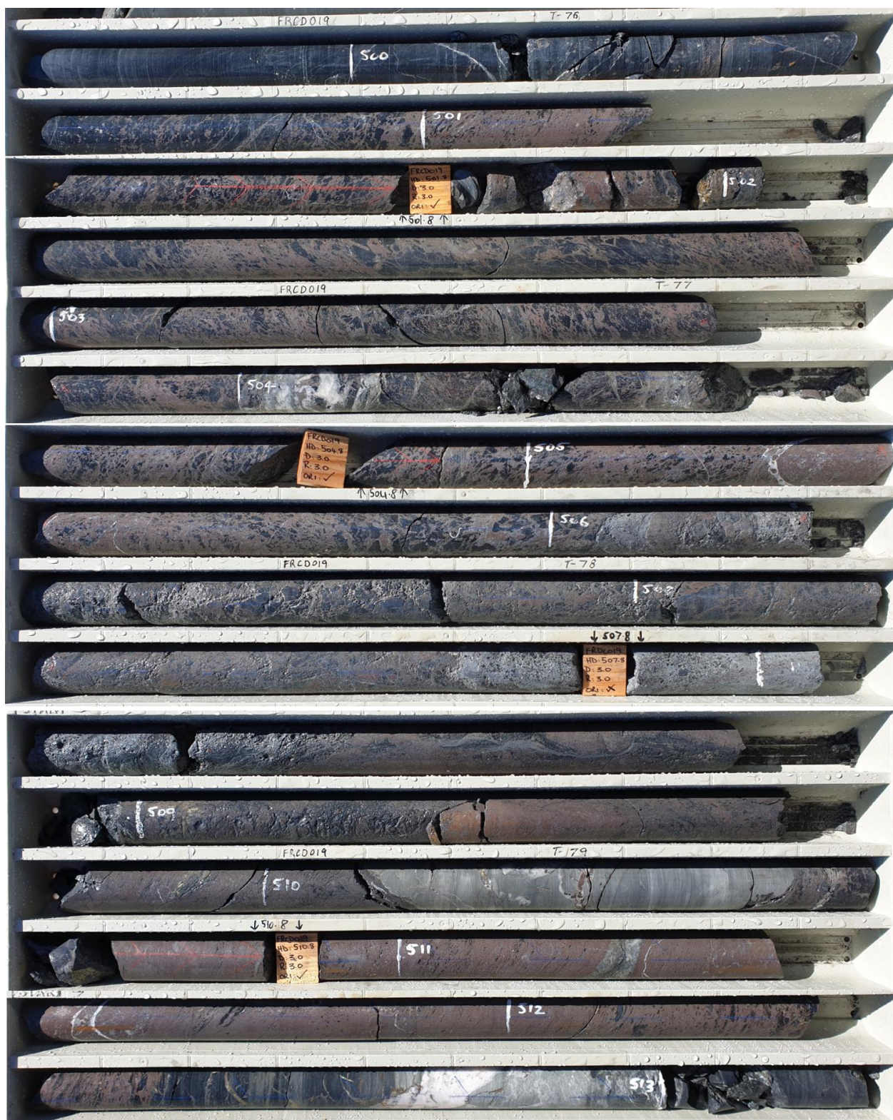
Figure 4. Composite photograph showing a zone in diamond hole FRCD019 with semi-massive and massive zinc-lead mineralisation (brown). Assays are pending for this hole.
