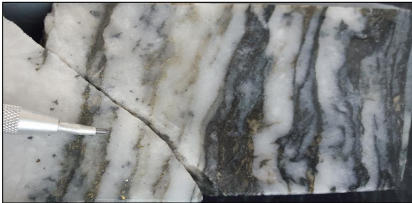
Figure 3: Laminated vein with 0.3 m at 230.0 g/t Au from 227.2 m (EVDD0048)
