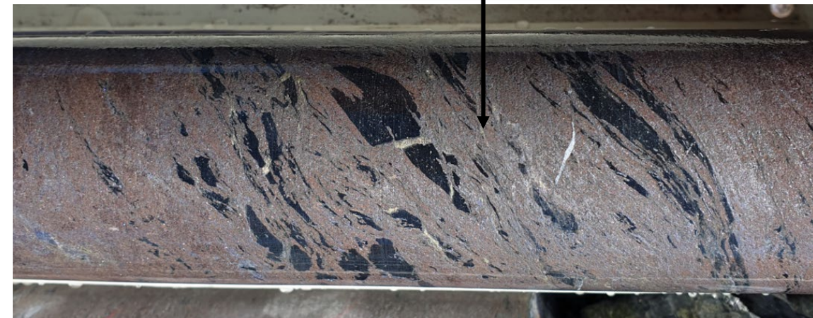
Strong Zn-Pb mineralisation intercepted in FRC019 drill core, ~490m below surface
