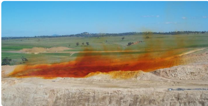
Blast fume using conventional explosives
