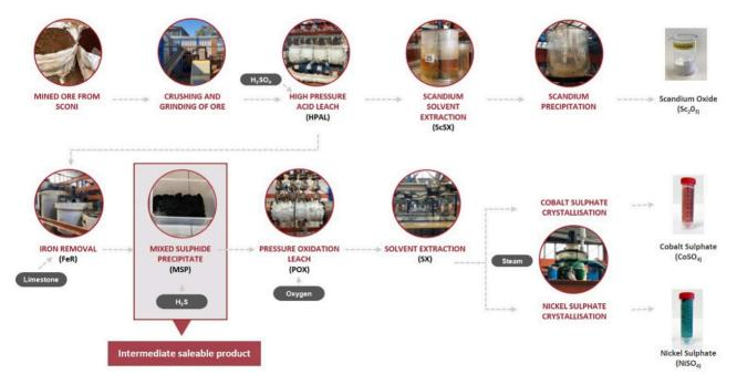
**Figure 4:** Australian Mines' proposed processing flowsheet that utilises proven, industry-standard technology, which has been comprehensively tested via the Company's demonstration-scale processing plant in Perth, Western Australia.
