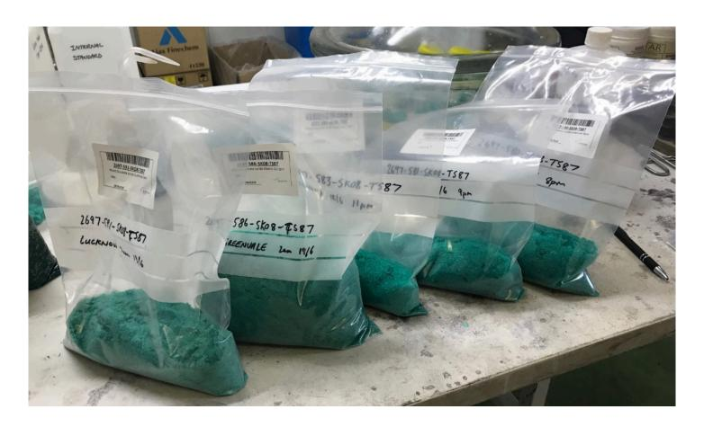
**Figure 5:** A sample of the battery-grade nickel sulphate produced from the company's demonstration plant located in Perth, Western Australia. In total, Australian Mines delivered 40 kilograms of battery-grade nickel sulphate (and 4 kilograms of cobalt sulphate) to electric vehicle battery manufacturer, SK Innovation, in July 2018.
