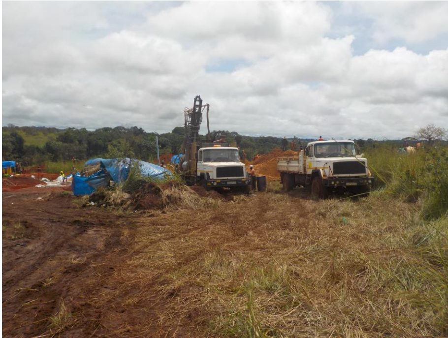
Photograph 1. Reverse Circulation drill rig setting up at drillhole PTRC002
