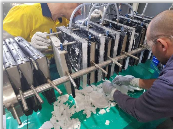
Removal of HPA pre-cursor from the filter
