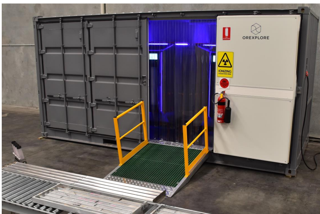
Fig 1. The Orexplore 20ft field container c/w three GeoCore X10 instruments and 120TB data management system.
