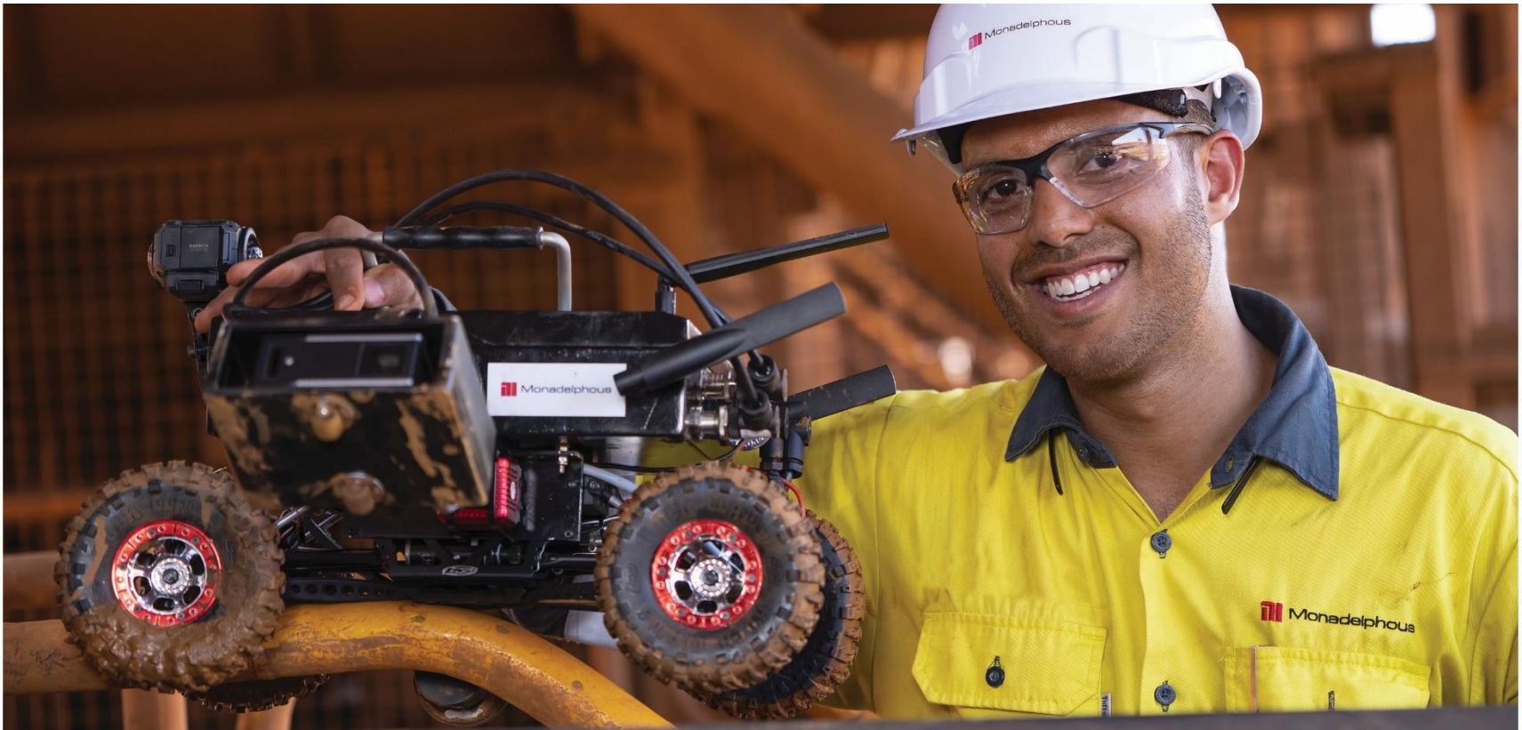
Monadelphous Mechatronics Engineer with our in-house developed skirt inspection robot.
