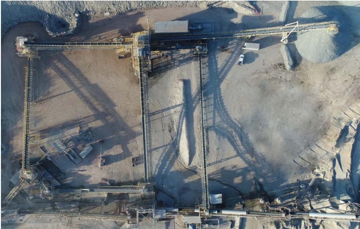
Figure 2: Nolans Processing Plant showing the beneficiation circuit. Reject material from beneficiation is located at the top right
