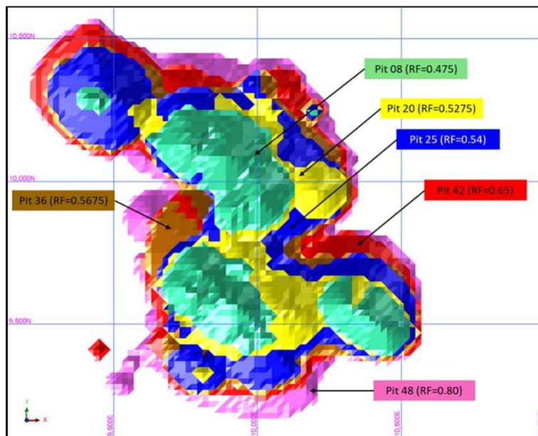
The resultant updated pit design shows some minor expansions over that developed for the DFS with minor expansions to the south, north-east and north-west, as well as a minor deepening. This comparison in final pit geometry is shown in the figure below.
