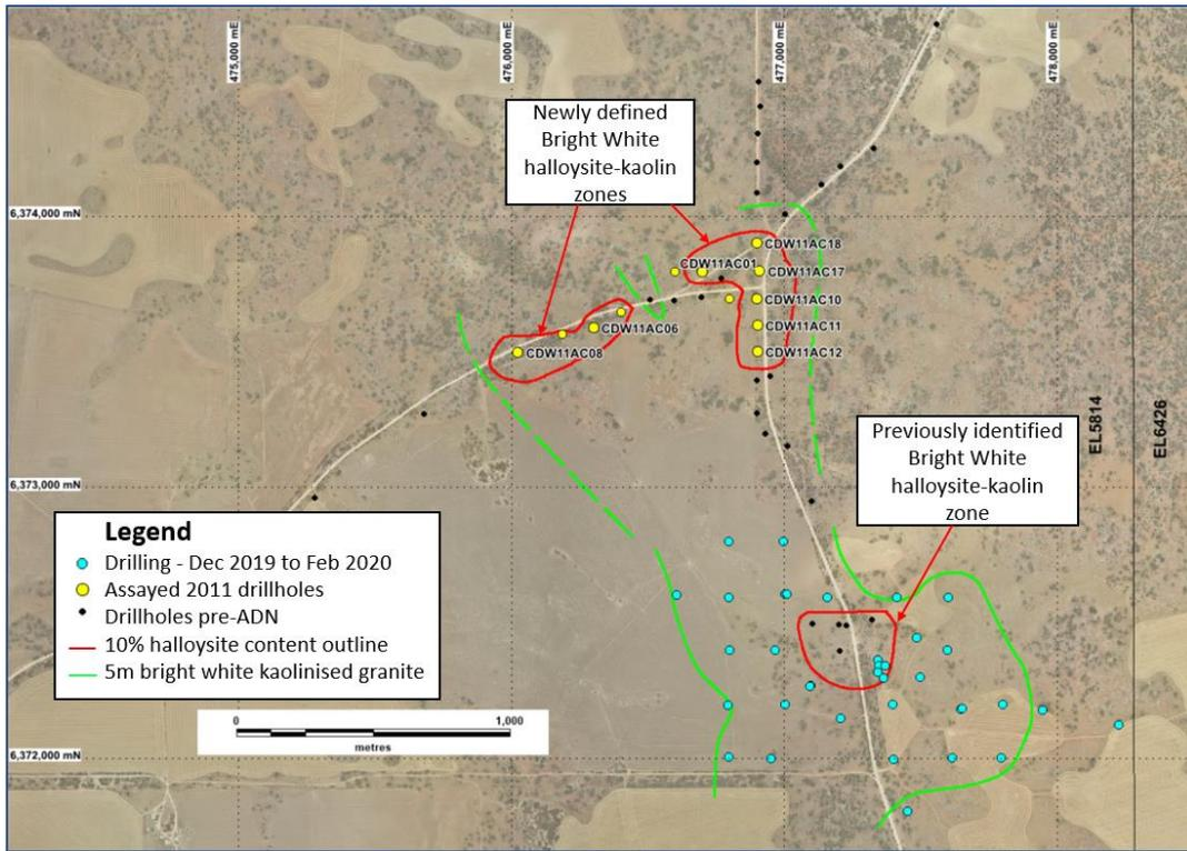
**Figure 2 : Dec 2019 to Feb 2020 drilling at Condoorie prospect with previous drill data's 10% halloysite content outline (note: recent drilling awaiting halloysite analyses) and an updated 5m Bright White kaolinised granite outline.**
