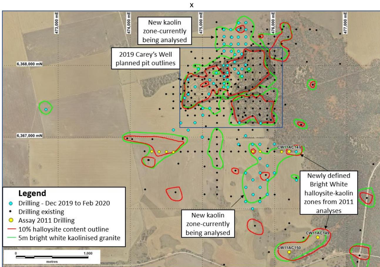
**Figure 4 : Dec 2019 to Feb 2020 drilling at Carey's Well deposit with previous drill data's 10% halloysite content outline (note: recent drilling awaiting halloysite analyses) and an updated 5m Bright White kaolinised granite outline.**
