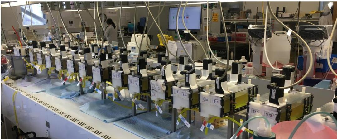
Figure 2: Side on view of SX mixer-settlers in the NdPr separation circuit during pilot operation
