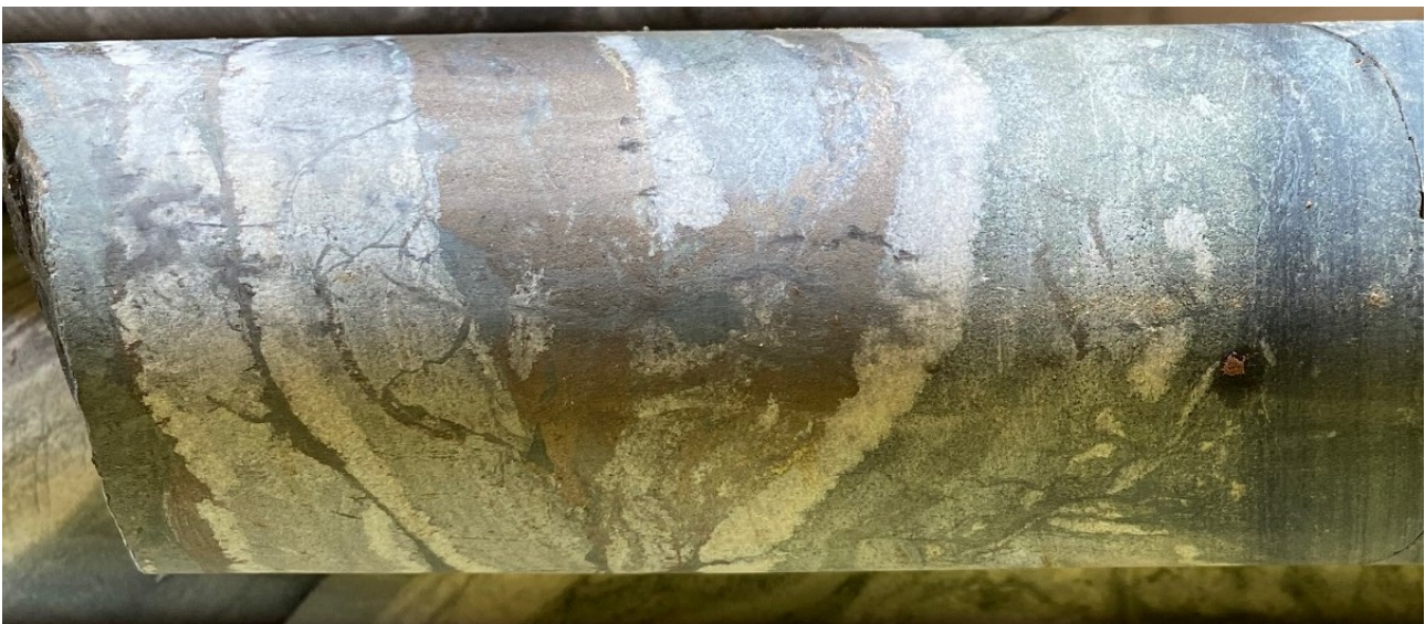
Figure 5: 15cm interval from 20LCDD001 with quartz-carbonate-pyrrhotite vein with carbonate-chlorite alteration selvage overprinting calc-silicate proto banded iron formation.
