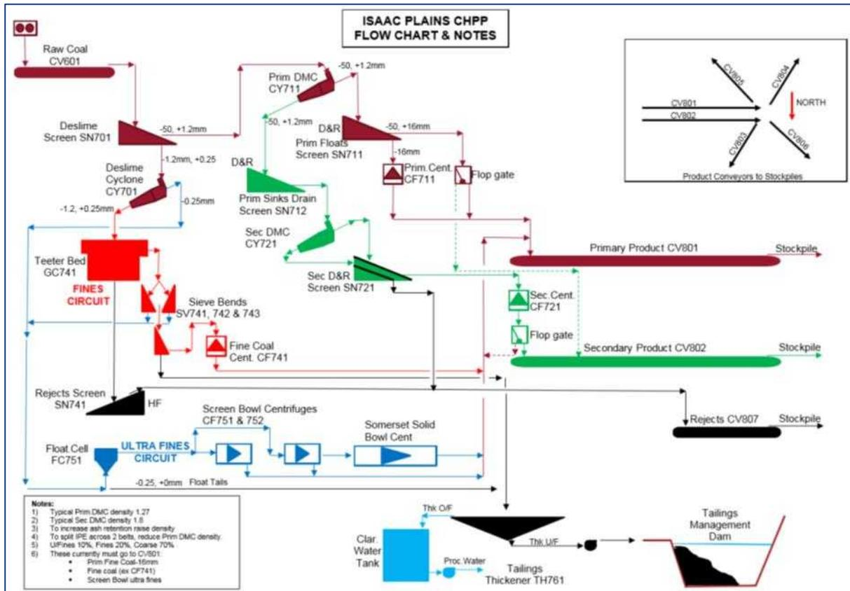
Rejects from the secondary DMC and TBS dewatered on screens and combined for disposal via a rejects conveyor to a rejects stockpile from where it is loaded into empty coal haulage trucks and returned to waste dumps.
