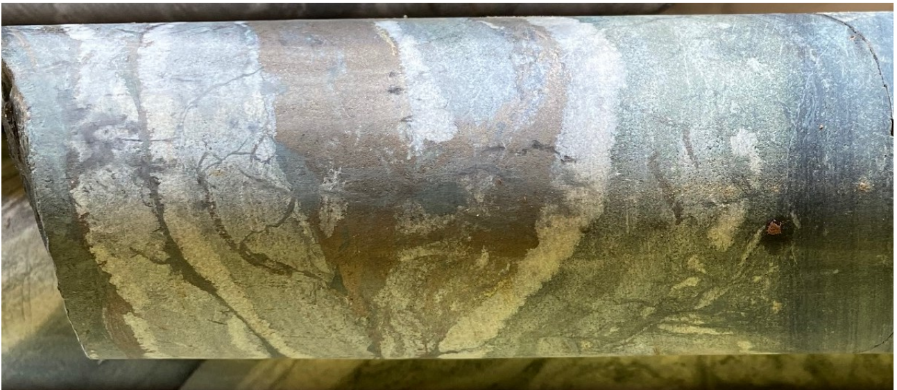
Figure 4: 15cm interval from 20LCDD001 with quartz-carbonate-pyrrhotite vein with carbonate-chlorite alteration selvage overprinting calc-silicate proto banded iron formation.
